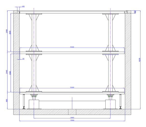
For lift travel of more than 5m we propose a solution with a detachable upper platform
